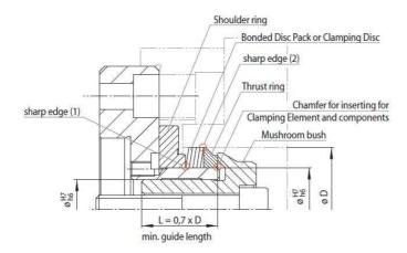
Push the RINGSPANN Clamping Discs / Disc Pack slightly oiled in / on the seating diameter. For an easier assembly the seating body can show a small guiding chamfer. The RINGSPANN Clamping Discs / Disc Pack are sitting on the seating diameter with a light pretension.! ^
